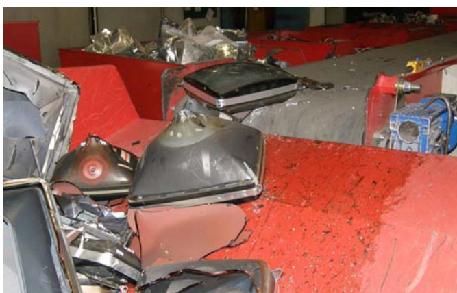
Figure 4. Poor handling leading to breakage and loss of fluorescent coatings during the dismantling process.
