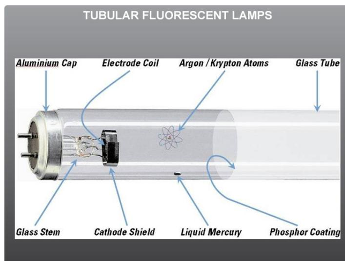
Fig 1: typical fluorescent tubular lamp (source: Lighting Industry Federation website)
