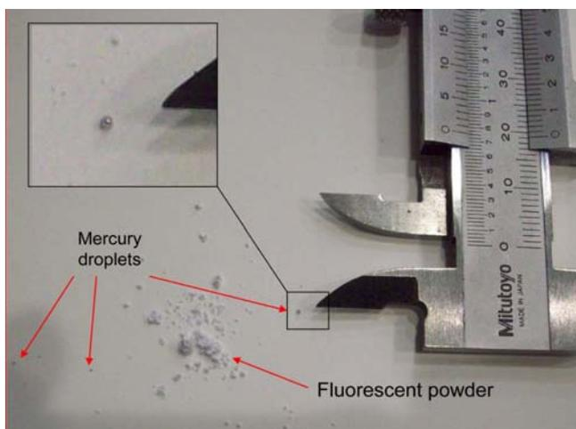
Fig 2: Mercury droplets and fluorescent powder released from a CCFL lamp breakage
