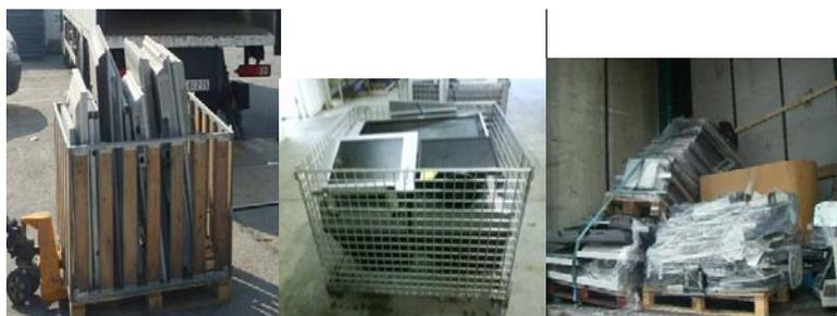
Fig 1: Good storage practice examples left and middle photos, compared to poor practice in right photo
