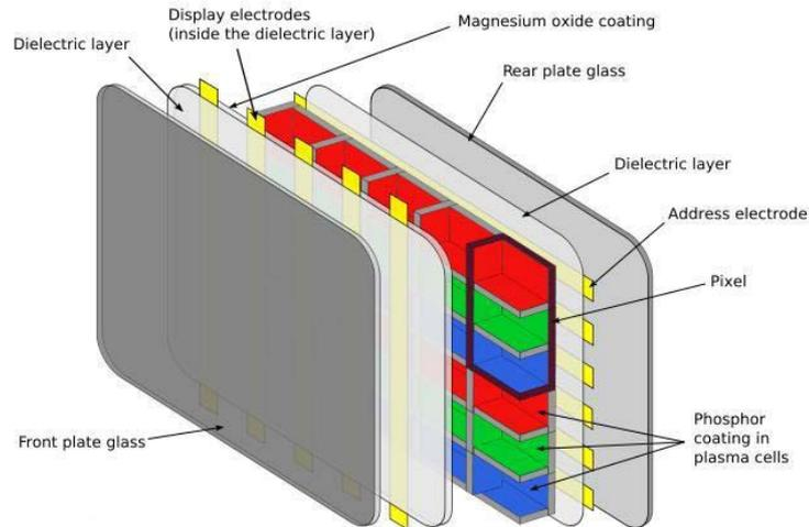
Fig 6: section through a typical plasma type display (source WRAP report, March 2009)
