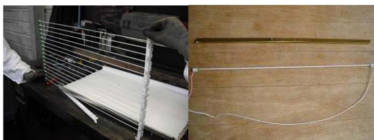
Fig 3: showing mercury backlights in typical TV and Laptop with protector strip (source WRAP report 2009)
