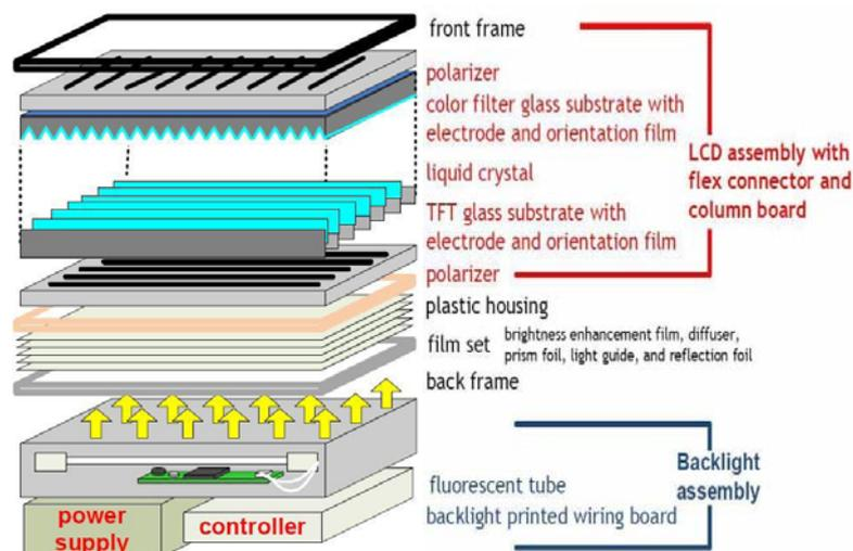
Fig 5: Section through a liquid crystal display (source WRAP report, March 2009)
