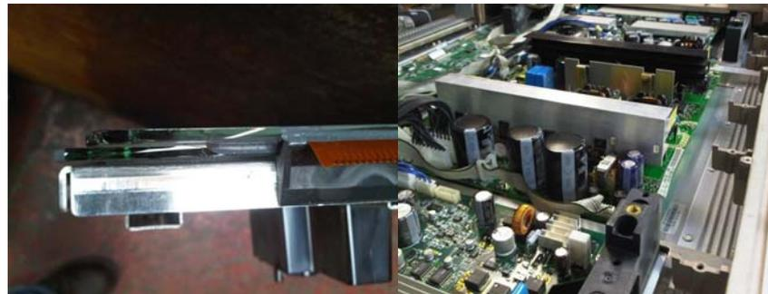
Fig 7: thick glass panels on plasma display and typically large circuit board with capacitors (source WRAP/ Bruce metals report 2009)
