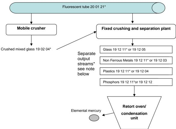
Figure 3: Typical process steps for fluorescent tube treatment (\*note- material specific codes for the crushed outputs can only be used after the initial hazardous waste assessment is completed and if the treatment results in an effectively separated non-hazardous material stream).
