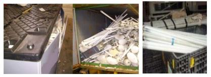
Figs 6, 7 & 8: Examples of poor lamp storage. Fig 6. corrugated container not assembled correctly (collar missing) therefore lamps not appropriately enclosed. Fig 7. lamps poorly stacked in oversized storage container leading to breakage. Fig 9. lamps not stored in appropriately sized enclosed container – risk of breakage.
