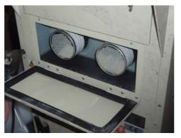
Figure 8 – example of mercury filters on small mobile crusher
