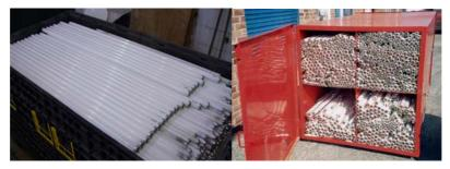
Figs 4 & 5: Good lamp storage practice - lamps neatly stored to minimise breakage
