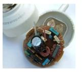
Fig 2 integrated ballast (source: http://commons.wikimedia.org/wiki/File:Elektronstarterp.jpg)
